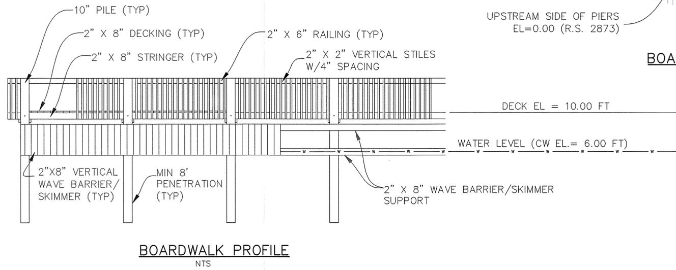
**BOARDWALK AND WEIR CROSS SECTION (SECTION C)**
