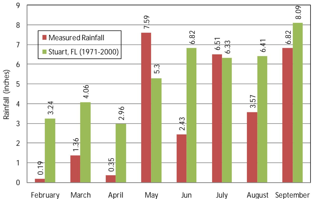
Figure 3-1. Comparison of Average and Measured Rainfall in the Vicinity of the Poppleton Creek Wet Detention Pond Site.
