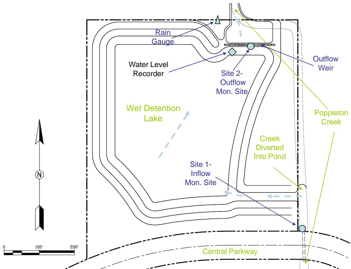
Figure 2-1. Locations for Monitoring Equipment at the Poppleton Creek Wet Detention Pond Site.
