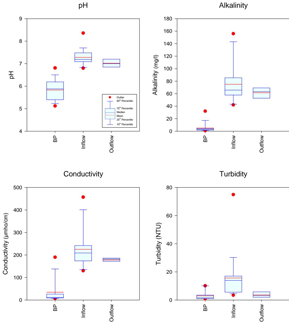
Figure 3-6. Summary of Statistical Variability in General Parameters Measured at the Poppleton Creek Wet Detention Pond Site.
