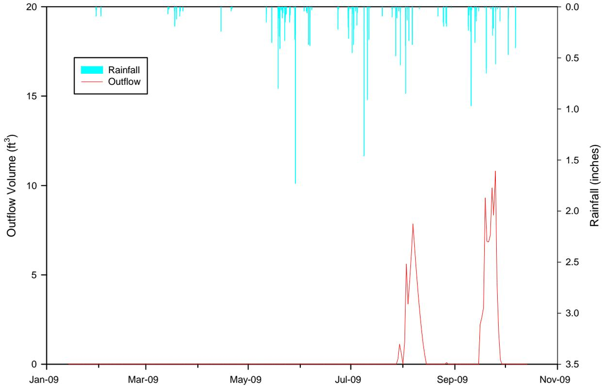
Figure 3-3. Outflow Hydrographs from the Poppleton Creek Wet Detention Pond from January 14-October 14, 2009.
