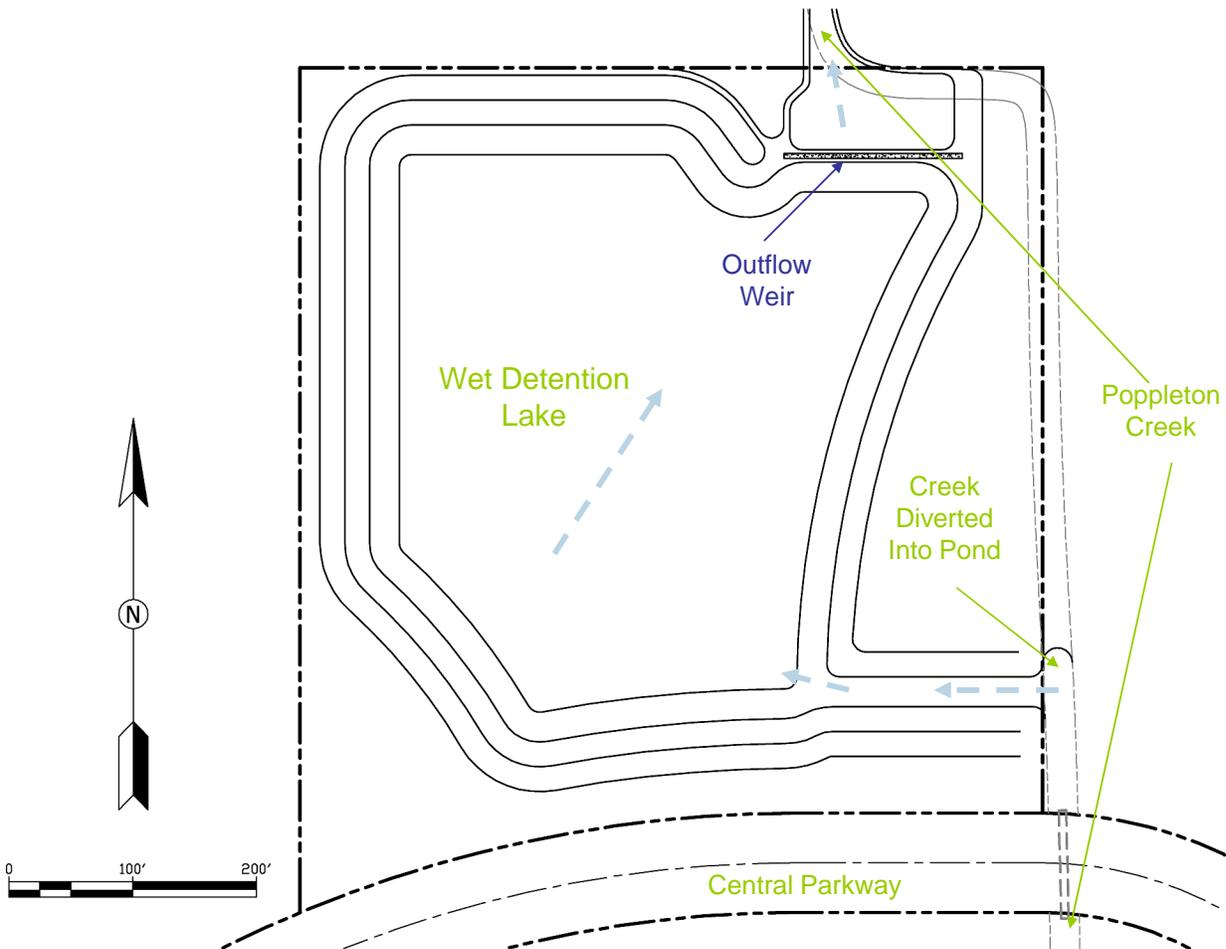
Figure 1-6. Schematic of the Poppleton Creek Detention Pond.
