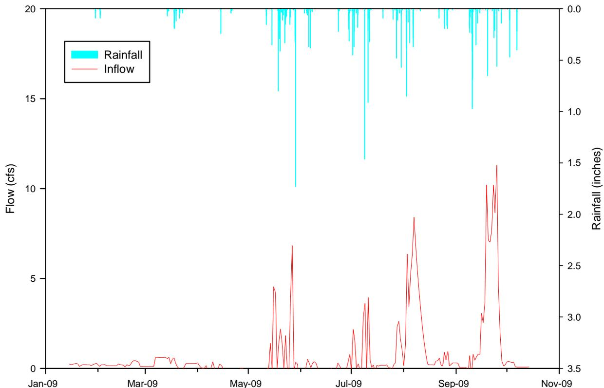
Figure 3-2. Inflow Hydrographs into the Poppleton Creek Wet Detention Pond from January 14-October 14, 2009.
