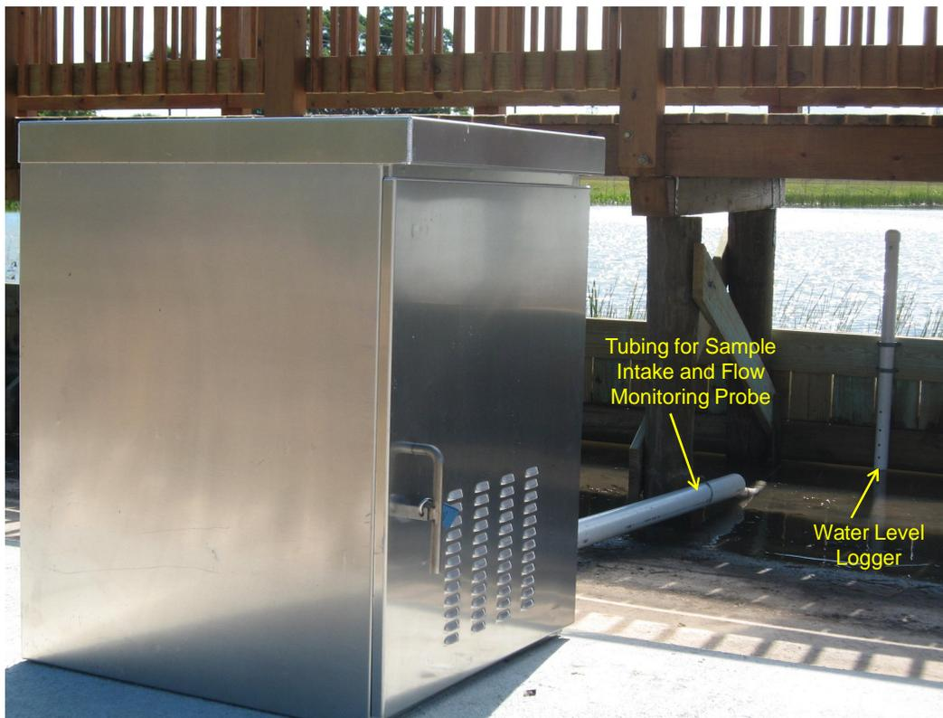
Figure 2-4. Autosampler Tubing and Water Level Logger.
