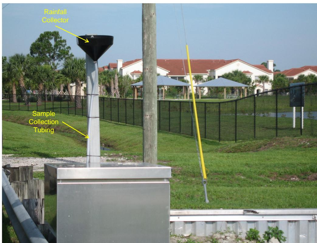
Figure 2-6. Bulk Precipitation Collector at the Inflow Monitoring Site.
